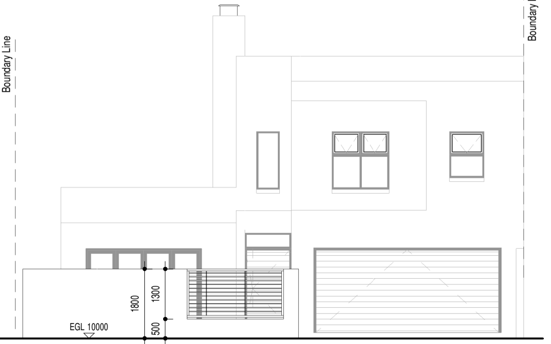
NORTH ELEVATION - BOUNDARY WALL 1 : 100
